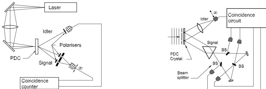
Figure 1 The experimental setups to observe the ‘quantum erasure’ effect. The one depicted on the left, by Walborn et al., uses polarisers (or quarter wave plates) to distinguish the signals passing through each slit. If no polarisers are present, then the usual diffraction pattern is observed. If orthogonal polarisers are placed before the slits, no diffraction pattern appears. But, when a polariser is placed before the idler signal and coincidences as a function of displacement are counted, they show either a fringe or anti fringe diffraction pattern. The setup on the right, by Kim et al., uses beam splitters to randomly select the various subsets.
